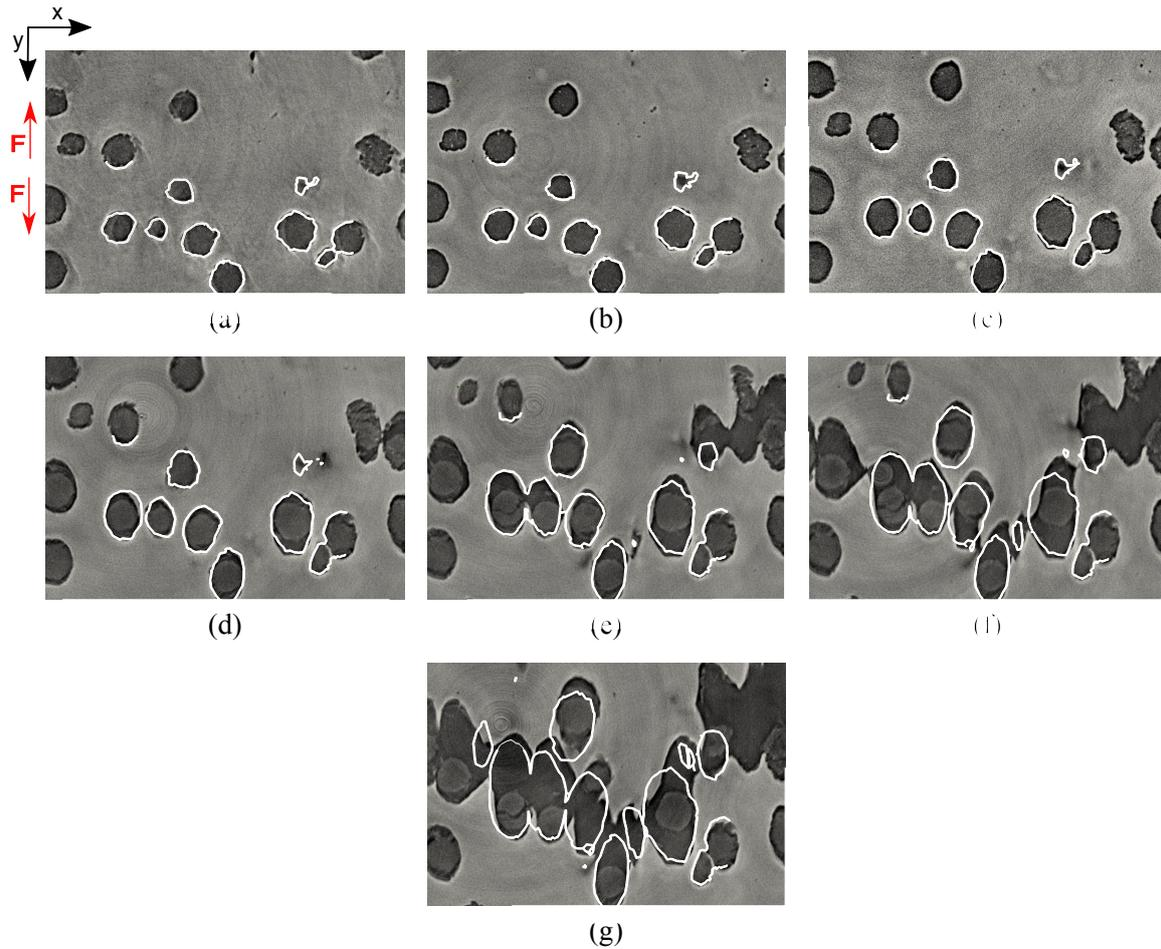
Figure 6.9 – Comparison between the void/matrix interface obtained by the FE simulation (thin white line) and the experimental images at a macroscopic displacement of: (a)  $0\ \mu\text{m}$ , (b)  $330\ \mu\text{m}$ , (c)  $578\ \mu\text{m}$ , (d)  $744\ \mu\text{m}$ , (e)  $868\ \mu\text{m}$ , (f)  $910\ \mu\text{m}$ , (g)  $950\ \mu\text{m}$ .
