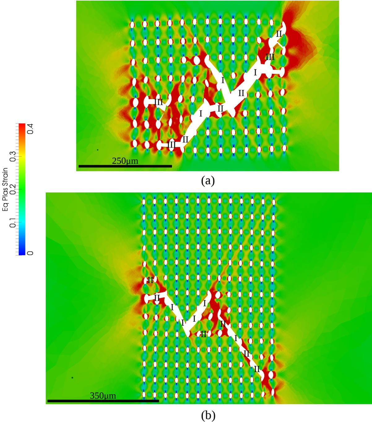
Figure 5.8 – Computational results for 7 and 13 lines of 13 holes at an engineering strain of: (a) 0.175, (b) 0.185.
