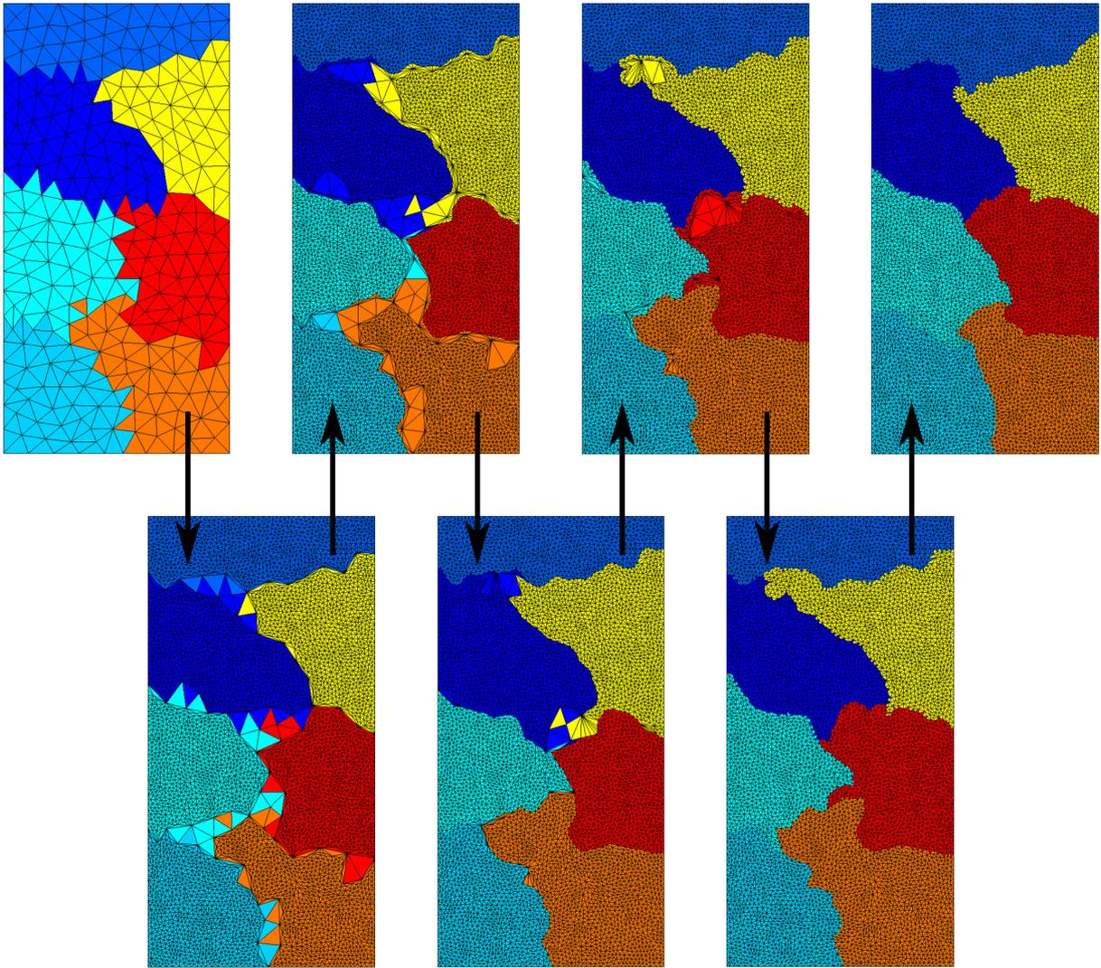
Figure 2.19 – Application of the parallel remeshing procedure to a 2D mesh, arrows pointing downward represent remeshing steps, while arrows pointing upward represent repartitioning steps. Partitions are distinguished by the coloring. Figure reproduced from [201].
