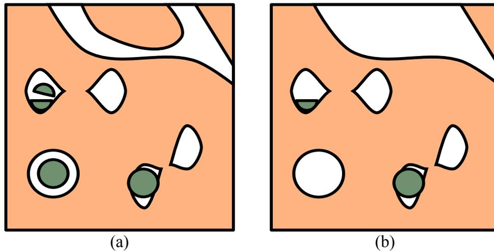
Figure 4.6 – Elimination of CCs of the solid phase that could lead to rigid body modes during mechanical solution: (a) initial microstructure with rigid body modes, (b) resulting microstructure after the numerical treatment.
