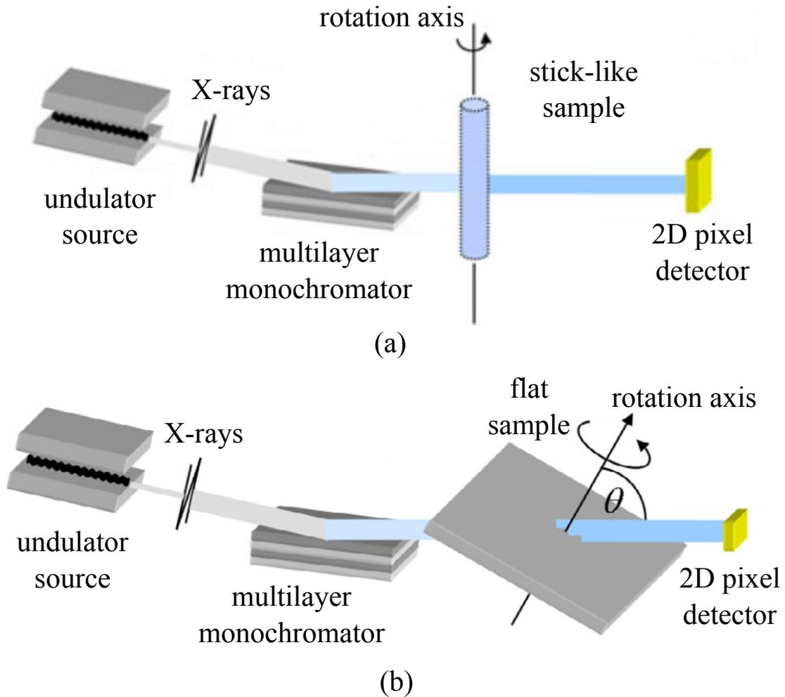
Figure 1.1 – Schematic drawing of: (a) a typical Synchrotron Radiation Computed Tomography (SRCT) setup, (b) a typical Synchrotron Radiation Computed Laminography (SRCL) setup,  $\theta \approx 60^\circ$ . Figures reproduced respectively from [63] and [22].
