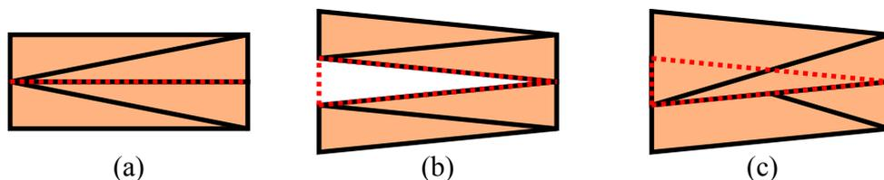
Figure A.3 – Cohesive elements with correct contact prediction: (a) initial mesh with cohesive element in red, (b) crack initiation, (c) inter-penetration of crack faces.
