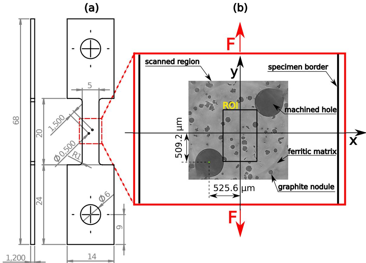
Figure 6.19 – (a) The sample geometry with the scanned region between the pin holes; (b) section of the reconstructed volume with ROI position.
