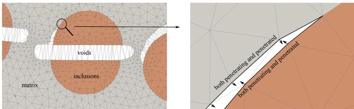
Figure A.1 – Contact situation in a 2D simulation with cracks.
