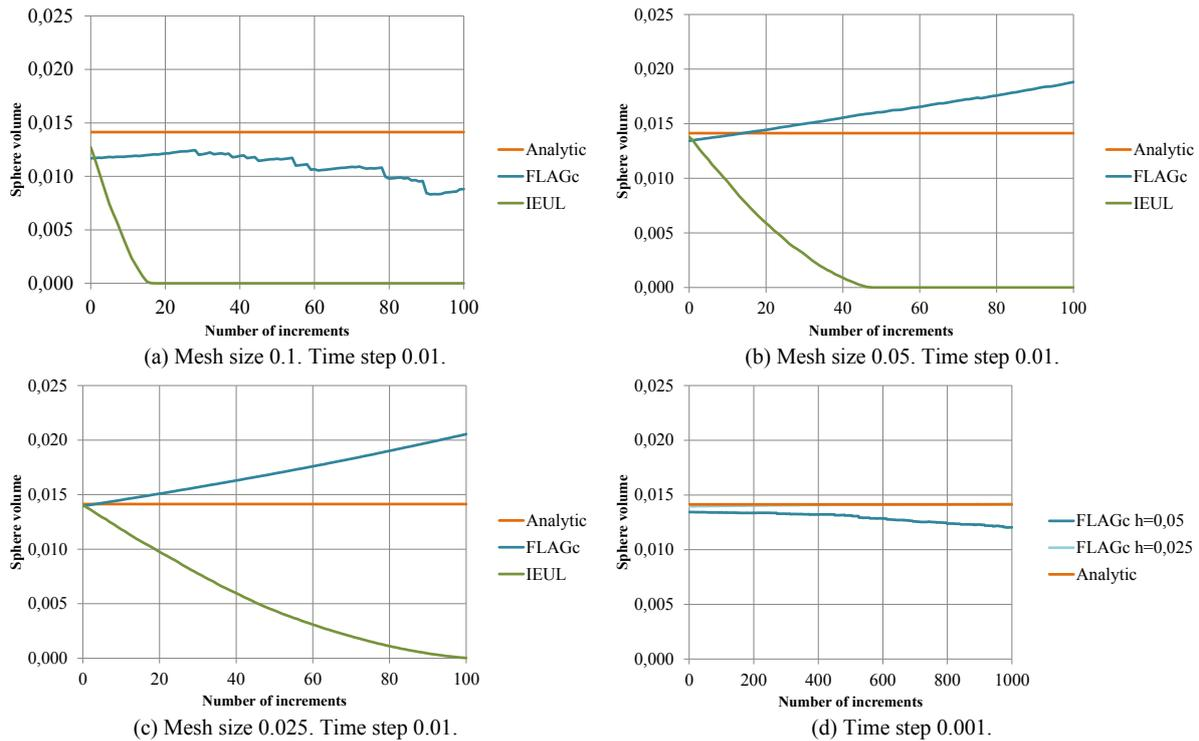
Figure 2.12 – Evolution of sphere volume during a full rotation using the reference time step and a mesh size of: (a) 0.1, (b) 0.05, (c) 0.025. (d) Evolution of sphere volume during a full rotation using a time step of 0.001.
