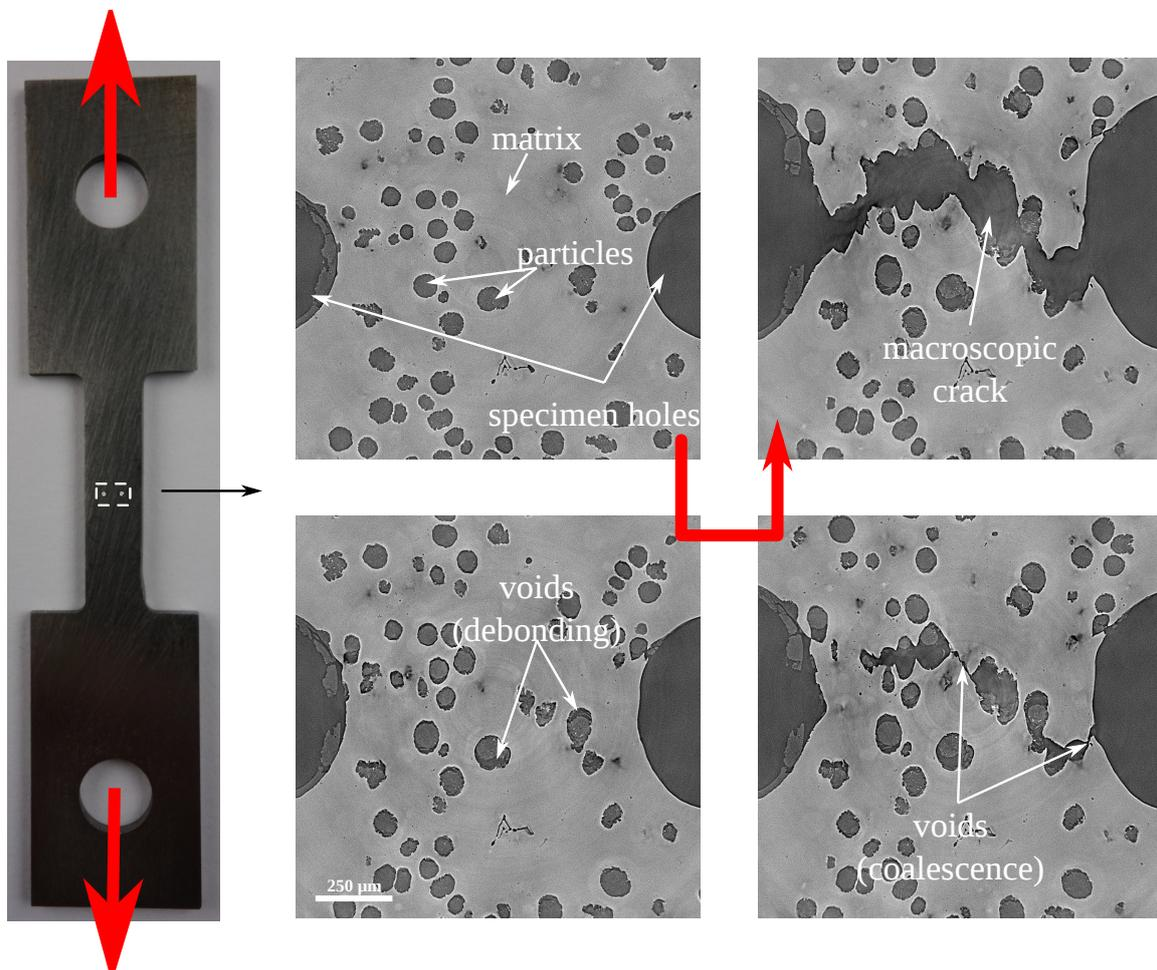
Figure 1 – Failure of a nodular cast iron specimen observed with Synchrotron Radiation Computed Laminography (SRCL) during an *in-situ* tensile experiment. The distance between the two holes is 1 mm. Courtesy of T. F. Morgeneyer.
