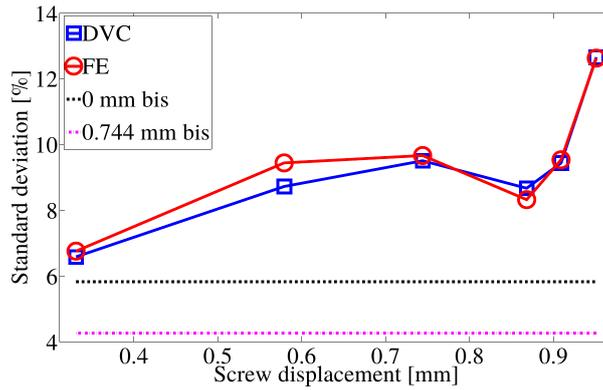
Figure 6.16 – Standard deviation for the dimensionless gray level residual fields for all loading steps (FE results obtained with  $h_2$  mesh). The standard deviations obtained for the repetition scans (0 mm bis) and rigid body motion scans (0.744 mm bis) are given for comparison (Paragraph 6.1.2.2.3).
