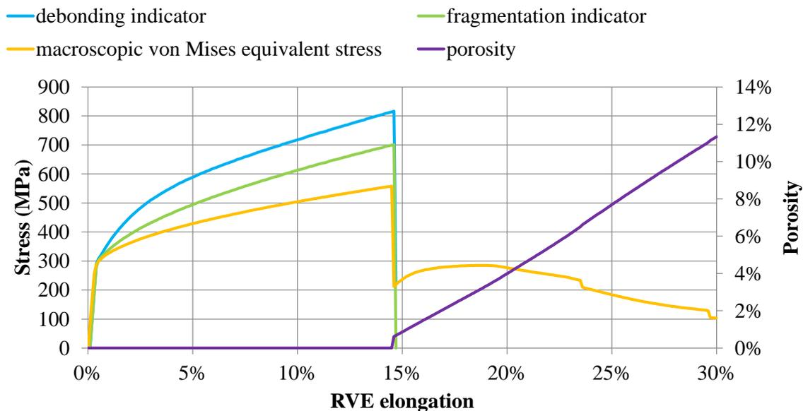
(b) Evolution of the particle debonding indicator  $\sigma_n$  (threshold at 1060 MPa), the particle fragmentation indicator  $\sigma_1^p$  (threshold at 700 MPa), the macroscopic von Mises equivalent stress  $\bar{\Sigma}$ , and the porosity  $f$ .
