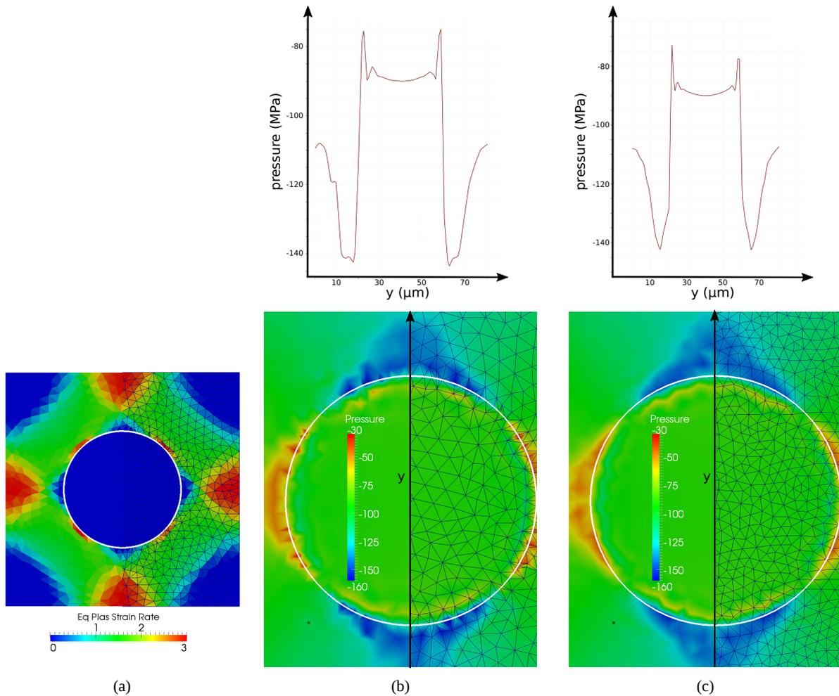
Figure 4.23 – Simulation result in 2D plane strain at 0.5 % of RVE elongation: (a) equivalent plastic strain rate using the fine meshing setting, (b) pressure field using the fine meshing setting, (c) pressure field using an initial mesh of uniform size  $2\ \mu\text{m}$  where the particle is initially meshed using a mesh generation software [192]. In (b,c), oscillations of the pressure at the matrix/particle interface are evidenced by the graphs.
