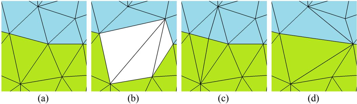
Figure 2.6 – Mesh adaptation with two phases: (a) initial patch, (b) illegal operation, (c) conform operation, (d) relaxation of the phase volumes conservation constraint.
