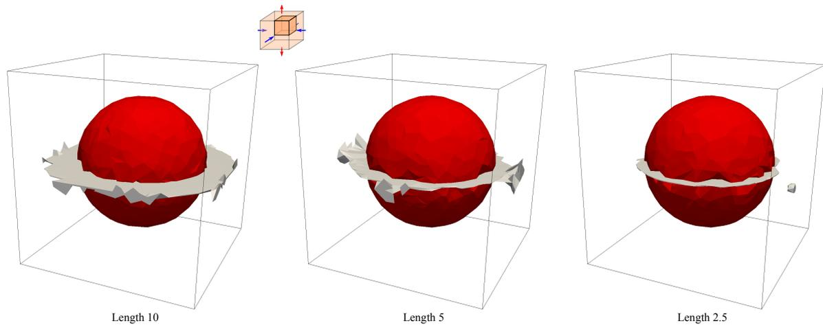
(a) Microstructures at the onset of particle fragmentation, with particle in red and voids in white.
