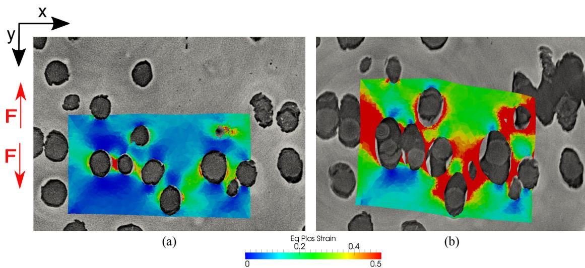
Figure 6.10 – Equivalent plastic strain obtained by the FE simulation superimposed with experimental images at a macroscopic displacement of: (a)  $578\ \mu\text{m}$ , (b)  $910\ \mu\text{m}$ .
