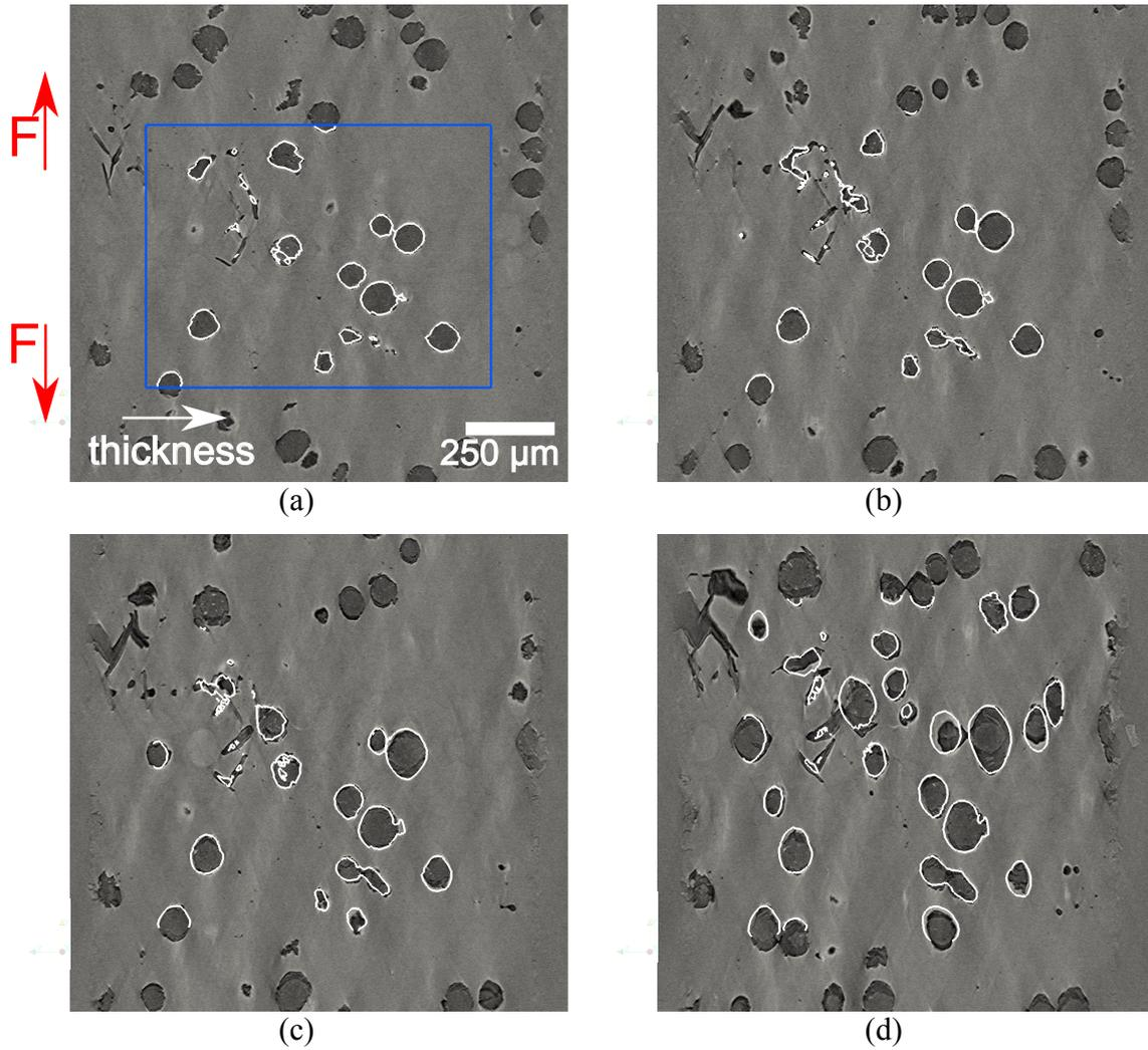
Figure 6.24 – ROI (blue line) calculation results using the DVC-FE approach comparing the numerical matrix/void interface (white line) with experimental images for the X midsection when: (a)  $\mathbf{u} = 0$  (undeformed state), (b)  $\mathbf{u} = 83 \mu\text{m}$ , (c)  $\mathbf{u} = 192 \mu\text{m}$ , (d)  $\mathbf{u} = 321 \mu\text{m}$ .
