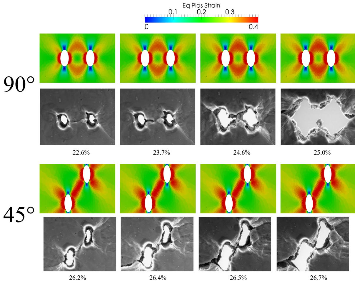
Figure 5.5 – Comparisons between computational results with no micro-cracking modeling and experimental observations at the last stages of void coalescence. Mentioned strains are engineering strains. Experimental images reproduced from Reference [83].
