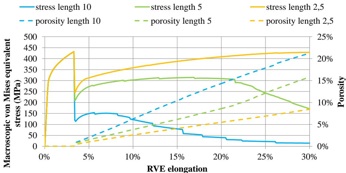
(b) Evolution of the macroscopic von Mises equivalent stress  $\bar{\Sigma}$  and the porosity  $f$ .Figure 4.15 – Sensitivity of the results with respect to the fragmentation crack extension length  $\ell^F$  in 3D.
