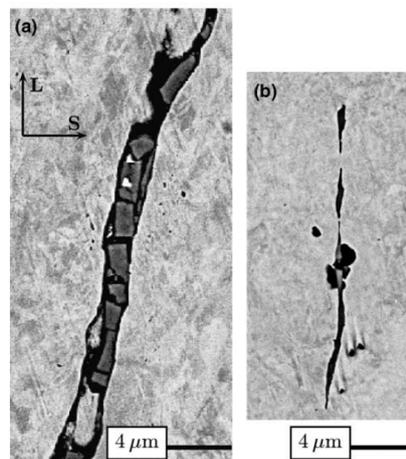
Figure 1.7 – Experimental observation of necklace coalescence during tensile tests (in the vertical direction) on a steel alloy. Figures reproduced from [88].
