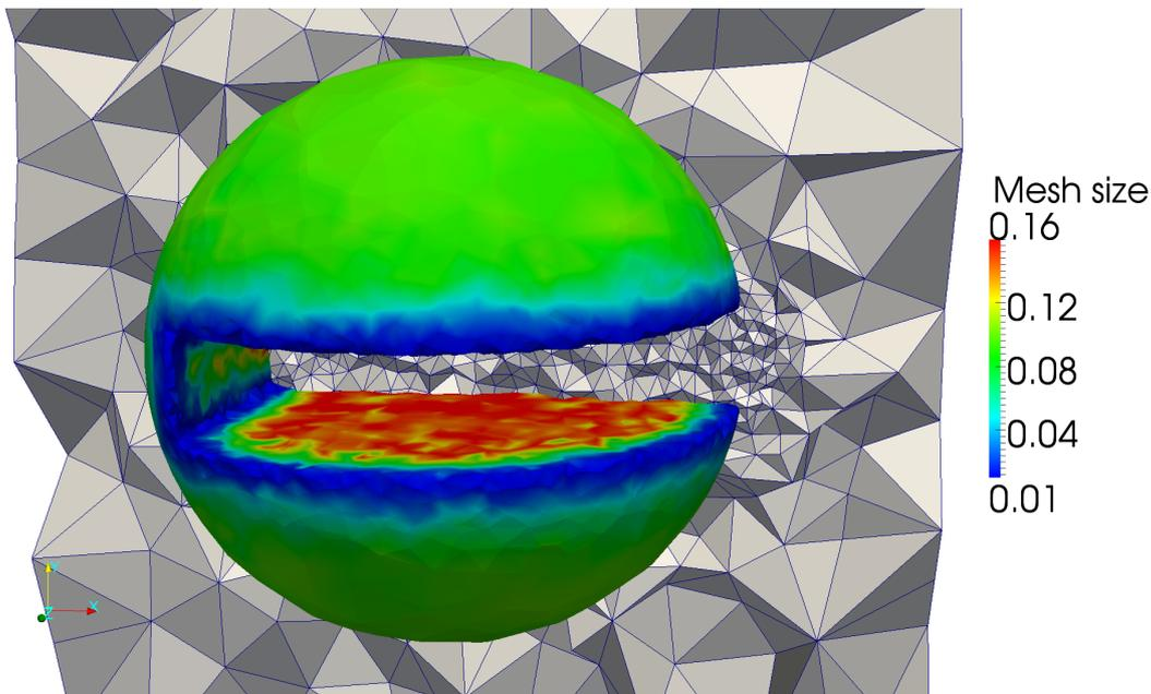
Figure 3.4 – Converged mesh for the Zalezak sphere test with  $h_c = 0.32$ . The interface is colored with respect to mesh size: regions in red have  $\lambda_{max} \rightarrow 0$  (mesh size is  $h_{max}$ ), regions in blue have  $\lambda_{max} \rightarrow \infty$  (mesh size is  $h_{min}$ ), and remaining regions are regular (mesh size depends on  $h_c$  and the local  $\lambda_{max}$ ).
