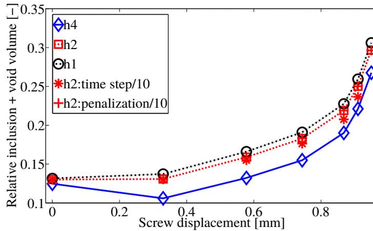
Figure 6.8 – Change of void volume (wrt. total ROI volume) with applied macroscopic displacement for various numerical parameters.
