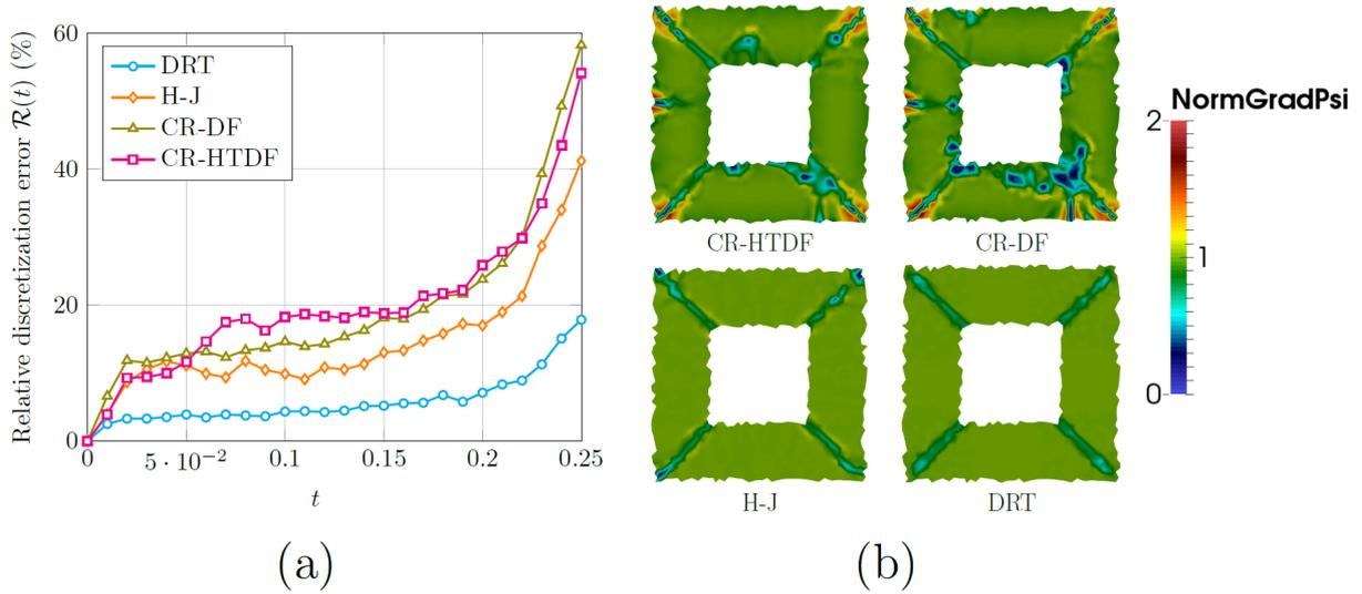
Figure 3.10 – Shrinking square test case: (a) relative discretization error  $\mathcal{R}(t)$  between the exact and computed distance functions around the interface  $\pm 5h$ , (b) values of  $\|\nabla\phi\|$  for each method at  $t = 0.08$ .
