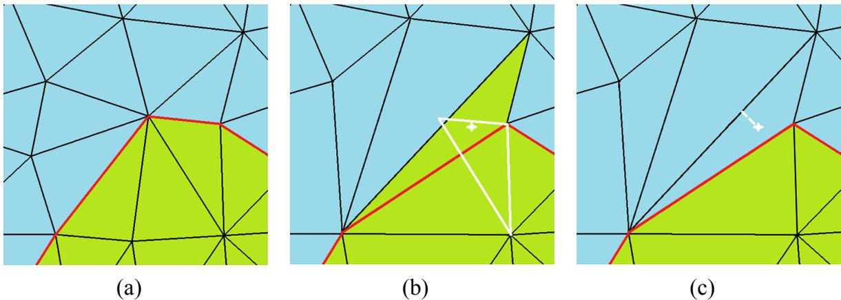
Figure 2.10 – Example of an incorrect transport of history variables: (a) initial mesh, (b) adapted mesh, (c) corrected transport. The two phases are colored in green and blue according to the  $H_i$  functions, and the interface is highlighted in red according to the  $\phi_i$  functions.
