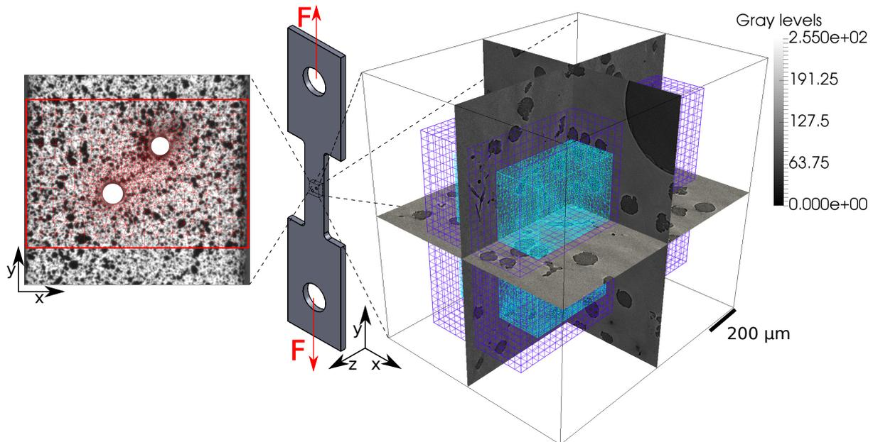
Figure 6.18 – Schematic view of the sample with zoomed region between the holes showing on the right: DVC (blue) and FE (cyan) meshes plotted over the corresponding cast iron microstructure in isometric view. On the left: surface image with speckle pattern and DIC mesh from test (B).
