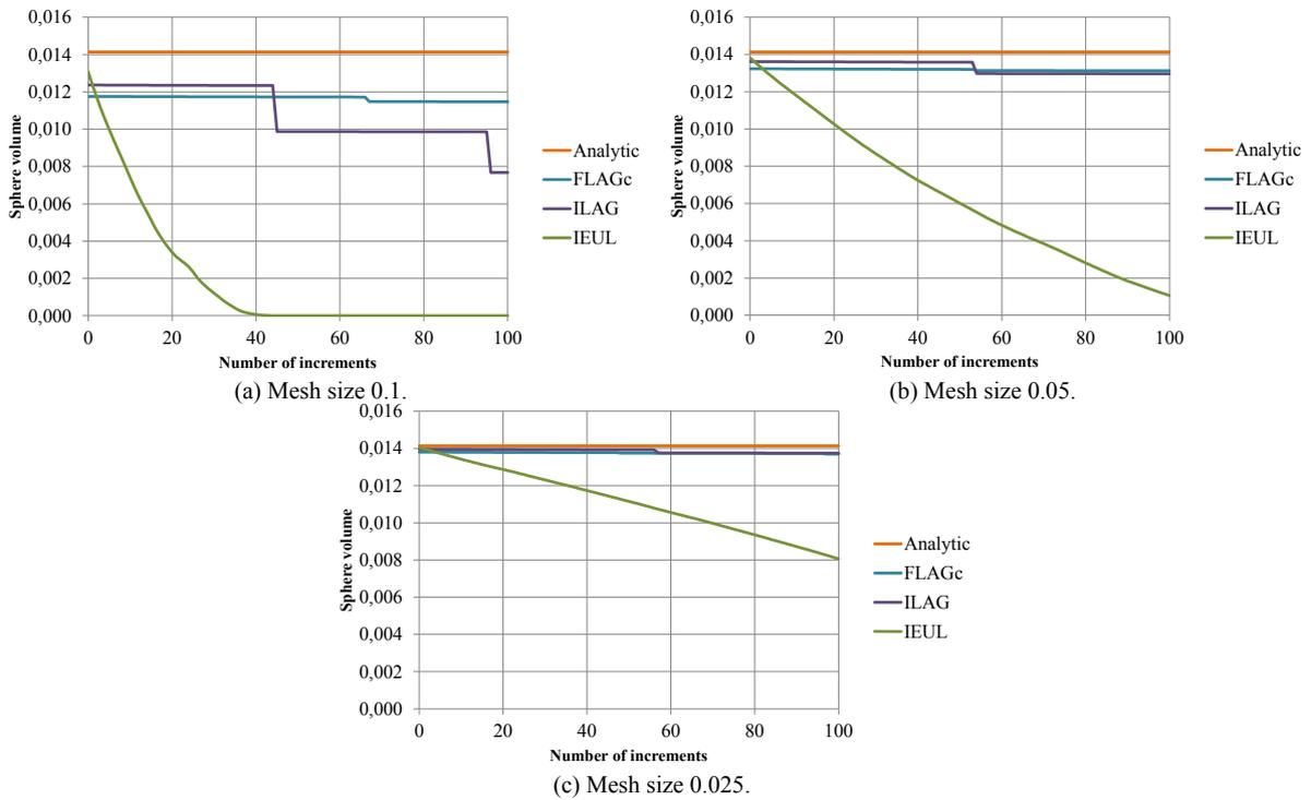
Figure 2.14 – Evolution of the volume of the sphere during its stretching. After 100 increments, the major diameter is doubled, while the other two are divided by  $\sqrt{2}$ . The mesh size is: (a) 0.1, (b) 0.05, (c) 0.025.
