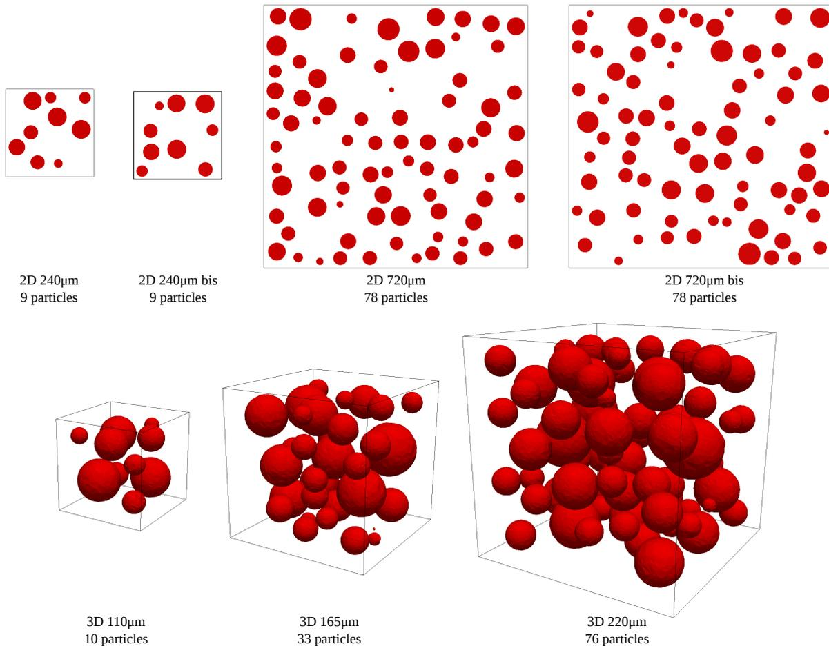
Figure 4.25 – Statistical RVEs used for the validation of RVE size. Particle volume fraction is close to 20 %, and particle radii follow a normal law of mean  $20\ \mu\text{m}$  and standard deviation  $5\ \mu\text{m}$ .
