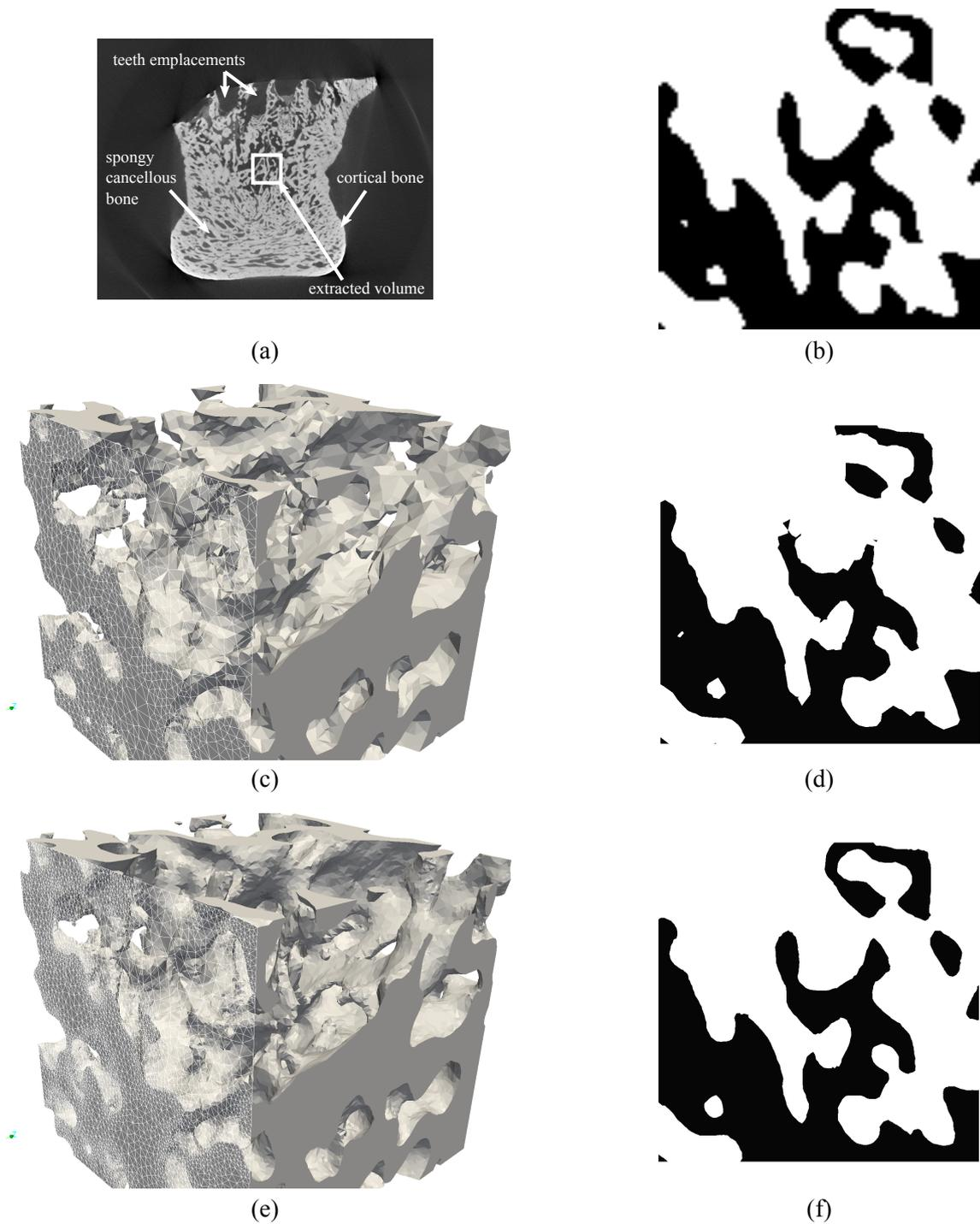
Figure 3.20 – Mesh generation from mandibular bone tomography images: (a) slice of the initial image, courtesy of Y. Tillier [225], (b) middle slice of the volume extracted from the initial image with cortical bone in black, (c) surface view of the cortical bone in the generated coarse mesh, (d) middle slice of the coarse mesh with cortical bone in black, (e) surface view of the cortical bone in the generated fine mesh, (f) middle slice of the fine mesh with cortical bone in black.
