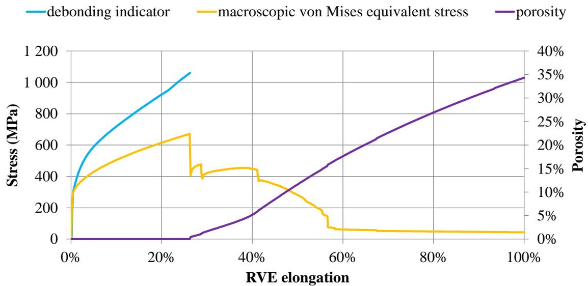
Figure 4.16 – Reference result in 2D plane strain, featuring only particle debonding, the fragmentation criterion being deactivated.
