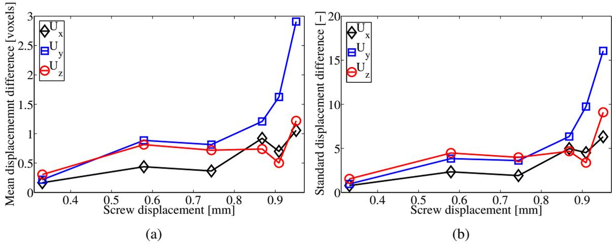
Figure 6.13 – (a) Mean values and (b) standard deviations (in %) of the difference between the measured simulated displacement fields for the FE mesh  $h_2$ . Standard deviations are normalized by the corresponding DVC uncertainties.
