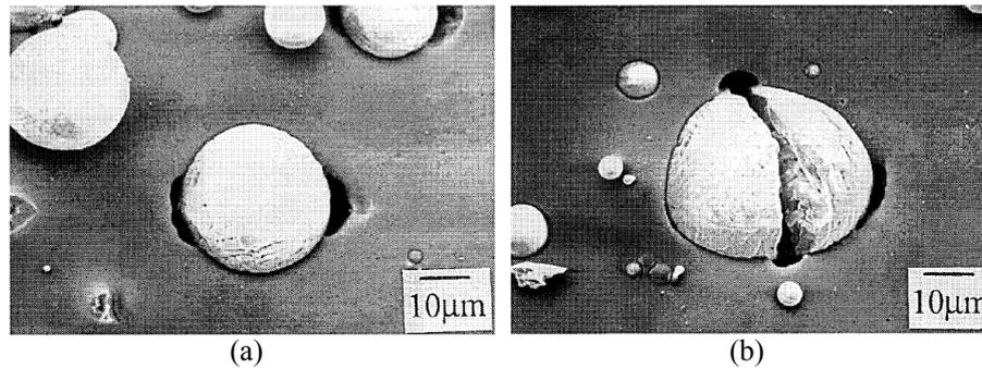
Figure 1.3 – SEM images of: (a) particle/matrix interface decohesion, (b) particle fragmentation. Loading was tension in the horizontal direction. Figures reproduced from [72].
