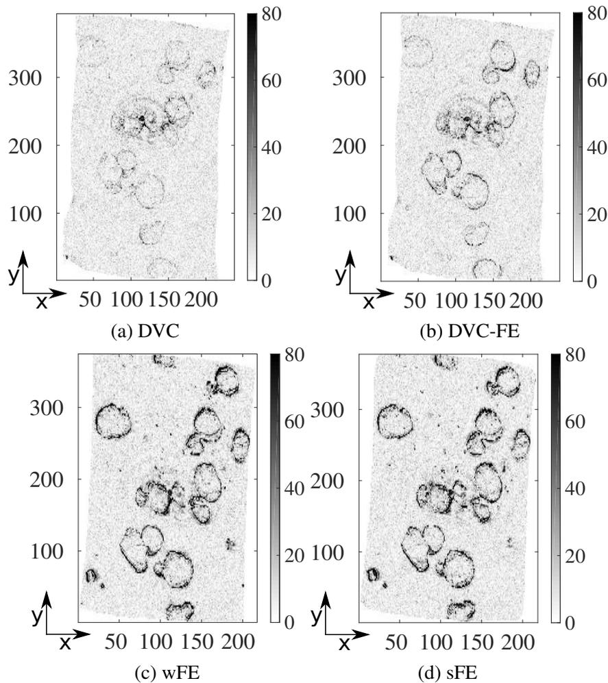
Figure 6.26 – Absolute gray level differences at the Z midsection after correction with DVC (a), DVC-FE (b), wFE (c) and sFE (d) displacements for the ninth loading step. Note that due to different rigid body motions for each simulation, the Z midsections slightly differ.
