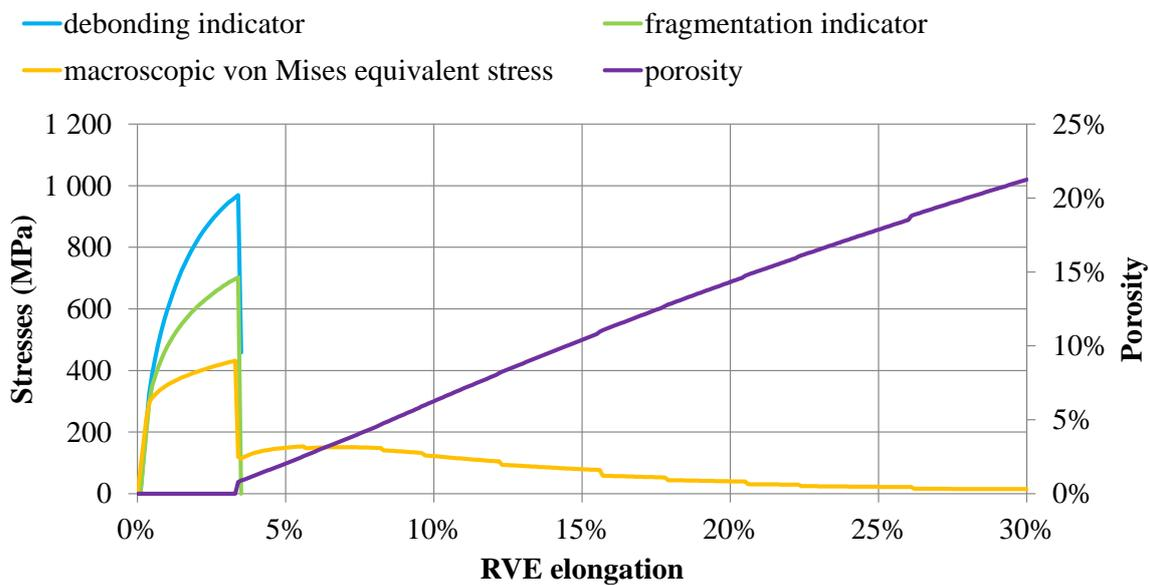
(b) Evolution of the particle debonding indicator  $\sigma_n$  (threshold at 1060 MPa), the particle fragmentation indicator  $\sigma_1^p$  (threshold at 700 MPa), the macroscopic von Mises equivalent stress  $\bar{\Sigma}$ , and the porosity  $f$ .
