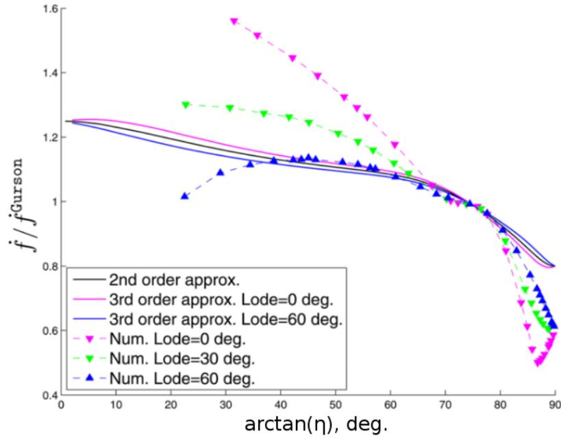
Figure 1.13 – Comparison between the porosity rate  $\dot{f}$  obtained using several analytic or numerical methods and Gurson's initial approximation  $\dot{f}_{Gurson}$ . These comparisons consider various stress states, represented by the angle  $\arctan \eta$  and the Lode angle  $\theta = \frac{27 \det(\Sigma')}{2 \bar{\sigma}^3}$ . Figure reproduced from [144].
