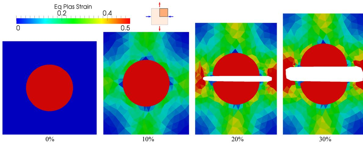
(a) Microstructure at different RVE elongations, with particle in red and voids in white.
