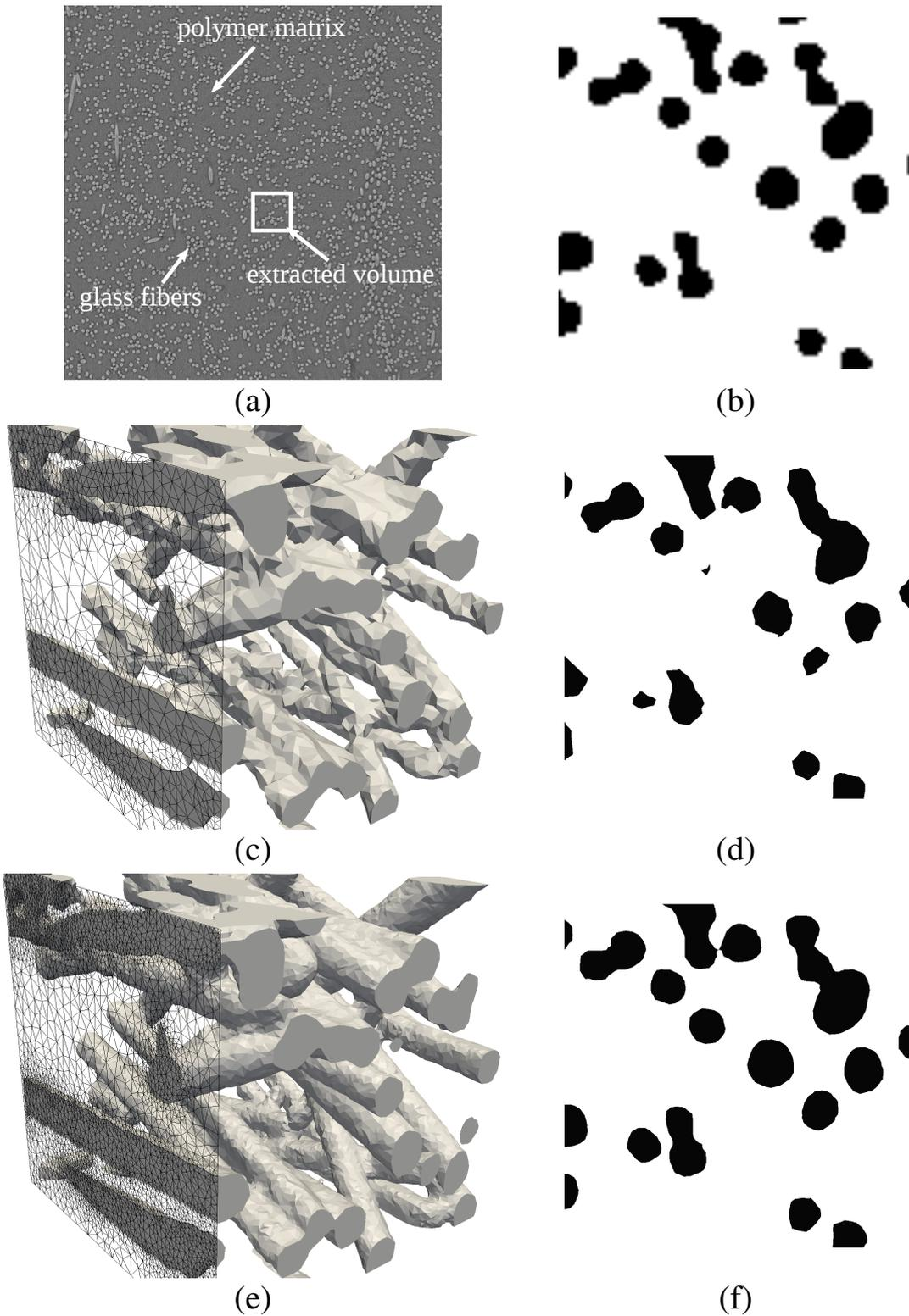
Figure 3.22 – Mesh generation from composite SRCT images: (a) slice of the initial image, courtesy of V. Fabre [226], (b) middle slice of the volume extracted from the initial image with glass fiber reinforcements in black, (c) surface view of fibers in the generated coarse mesh, (d) middle slice of the coarse mesh with glass fiber reinforcements in black, (e) surface view of fibers in the generated fine mesh, (f) middle slice of the fine mesh with glass fiber reinforcements in black.
