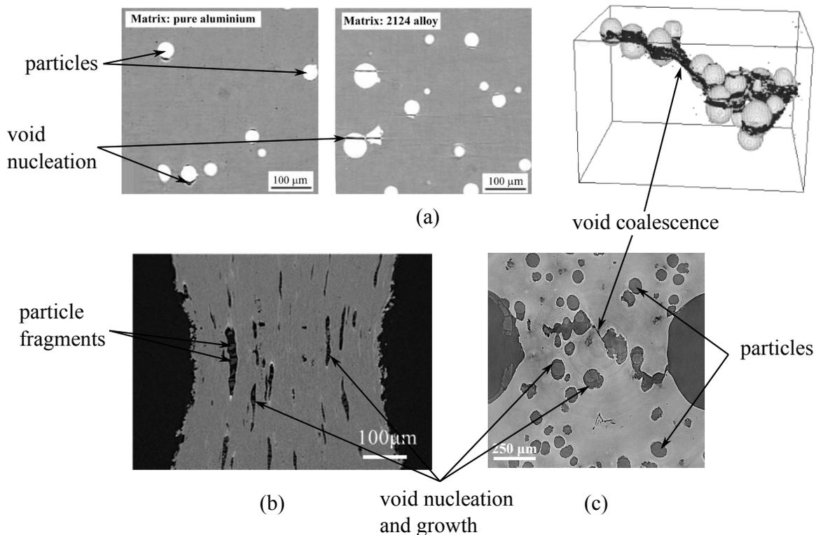
Figure 1.2 – X-ray images: (a) Computed Tomography (CT) images of aluminum alloys reinforced with zirconia/silica ( $ZrO_2/SiO_2$ ) particles, figures reproduced from [66], (b) CT image of a steel sample containing manganese sulfide (MnS) particles, figure reproduced from [67], (c) Computed Laminography (CL) image of nodular cast iron, courtesy of T. F. Morgeneeyer.
