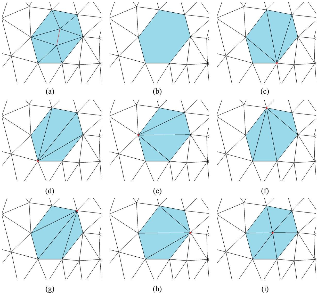
Figure 2.8 – Example of patch at the wide gathered neighboring of an edge: (a) initial patch, (b) external faces extraction, (c-i) candidates.
