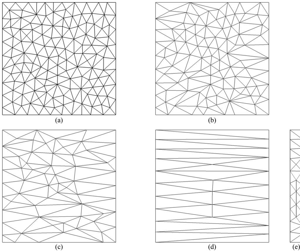
Figure 3.2 – Metric-driven mesh adaptation applied to a 2D anisotropic example: (a) initial mesh, (b,c) progressive adaptation, (d) final mesh, (e) final mesh as the remesher sees it.
