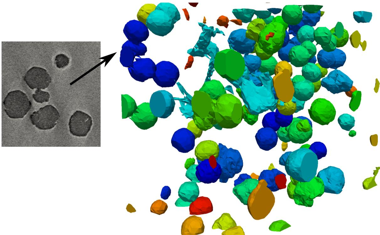
Figure 3.23 – Mesh generation from nodular cast iron SRCL images, final mesh with CCs identification. The nodules pointed out by the arrow are tagged with the same identifier because they are very narrow and in contact at some points in the initial X-ray image.
