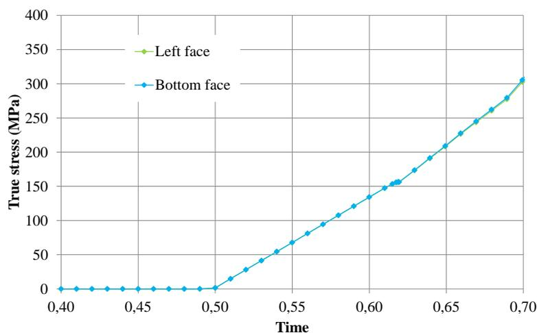
Figure A.9 – True stress measured at the left and bottom faces of body 1 for the 2D contact test case.
