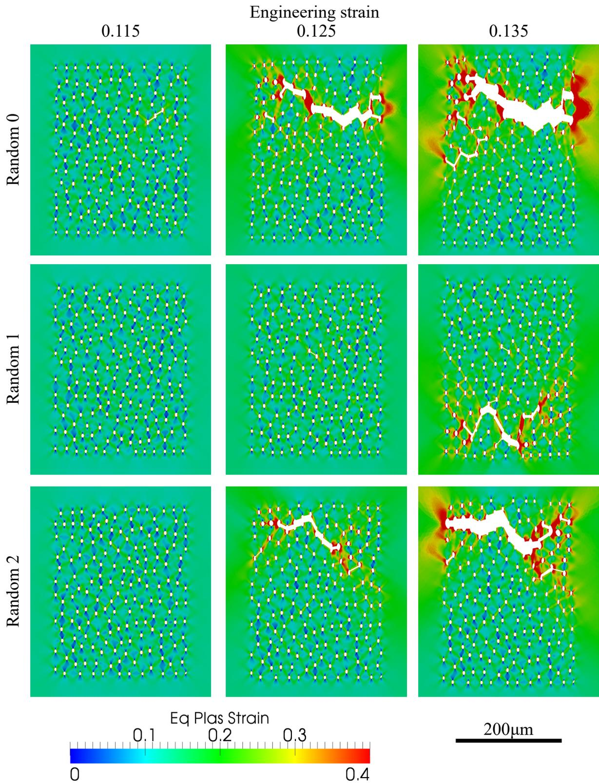
Figure 5.13 – Computational results for random hole arrangements at different engineering strains.
