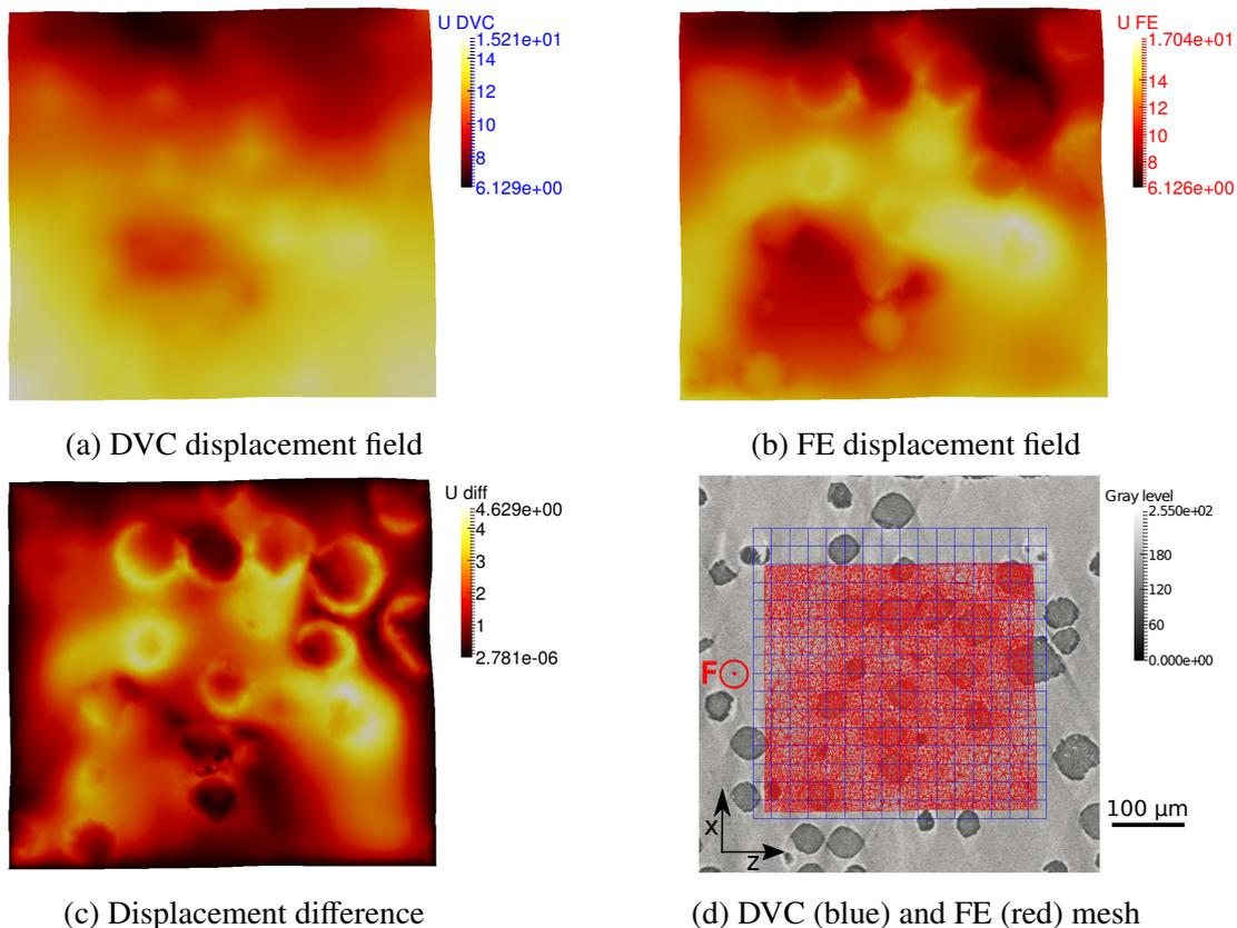
Figure 6.12 – Section normal to  $y$ -direction: (a) DVC displacement field magnitude, (b) FE displacement field magnitude, (c) absolute difference between them and (d) DVC and FE meshes for the third loading step. All reported values are expressed in voxels ( $1\text{ voxel} \leftrightarrow 1.095\ \mu\text{m}$ ) and correspond to the FE mesh  $h_2$ .
