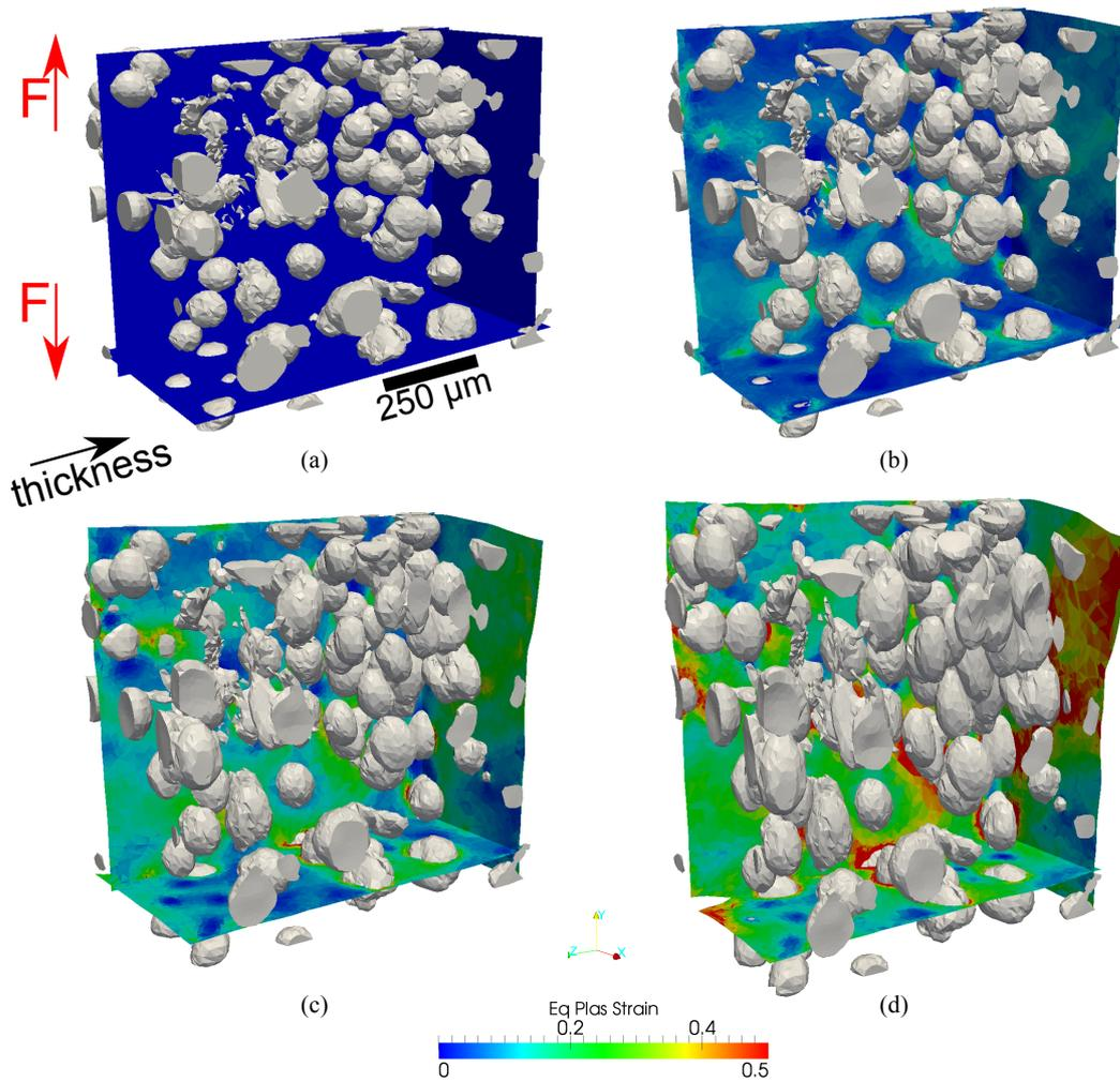
Figure 6.23 – ROI calculation results using the DVC-FE approach showing the 3D meshed voids and the equivalent plastic strain on sections when: (a)  $u = 0$  (undeformed state), (b)  $u = 83 \mu\text{m}$ , (c)  $u = 192 \mu\text{m}$ , (d)  $u = 321 \mu\text{m}$ .
