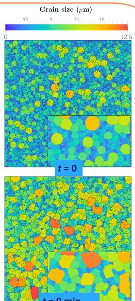
Expression obtained for the limiting grain size:  $\langle R_f \rangle = 0.362 \langle R_0 \rangle f_{gb}^{-0.853(r_p/\langle R_0 \rangle)^{0.428}}$
