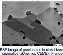
BSE image of precipitates in nickel based superalloy (S.Vernier, CEMEF, France)
