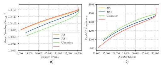
**Figure 14.** Evolution of different parameters as a function of the number of grains, for the 2D heterogeneous GG test case simulated with the TRM model: (a) total grain boundary energy  $E_{\Gamma}$  and (b) total length of GBs.
