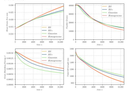
**Figure 13.** Evolution of different parameters as a function of time, for the 2D heterogeneous GG test case simulated with the TRM model: (**top-left**) mean grain size pondered by surface, (**top-right**) number of grains, (**bottom-left**) total grain boundary energy  $E_{\Gamma}$  and (**bottom-right**) total lenght of GBs.
