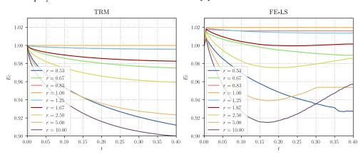
**Figure 7.** Triple junction test case: evolution of the normalised total grain boundary energy  $E_{\Gamma}$  for the (**left**) TRM and (**right**) LS-FE models. The plotted data for the LS-FE model was taken from [8].
