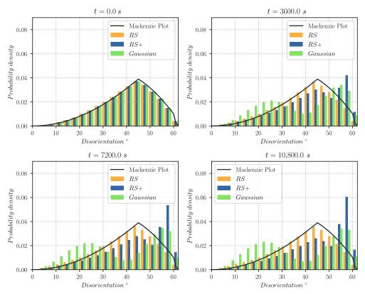
**Figure 10.** Probability density plot of the disorientation angle weighted by GB length, for the cases using the Gaussian, RS, and RS+ functions for the computation of the GB energy  $\gamma$ , and for different times. Each class of data contains the results of four different initial states representative of the same initial grain size distribution.
