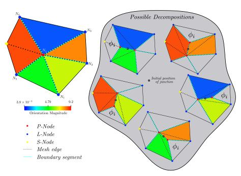
**Figure 1.** Possible decompositions of a fifth-order MJ. Data regarding the orientation of each grain are given. One possible decomposition for every phase involved is depicted. The decomposition of a 5th order MJ results in a 4th order MJ and a third-order MJ.
