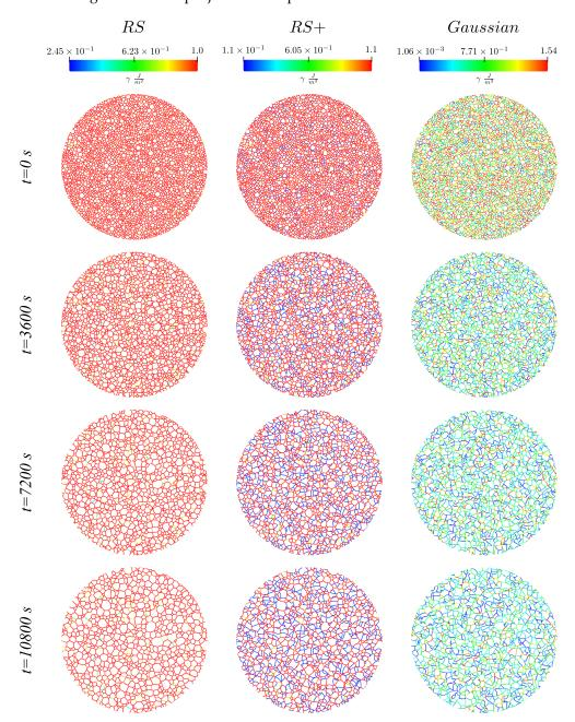
**Figure 9.** Examples of the evolution of the microstructure, from top to bottom as a function of time, and using the functions from right to left: RS, RS+, and Gaussian. A much higher heterogeneity is found in the cases using the Gaussian and RS+ functions. These figures illustrate the presence of stable high-order multiple junctions.
