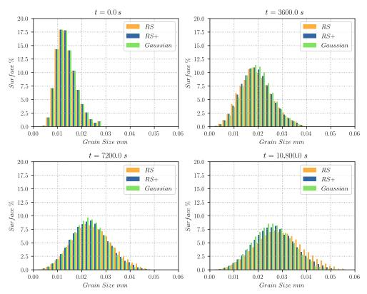
**Figure 12.** Grain size distributions weighted by surface using various functions for the computation of the GB energy  $\gamma$ . The distributions are given for every hour of thermal treatment. Each class of data contains the results of four different initial states representative of the same initial grain size distribution.
