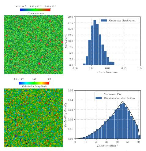
**Figure A1.** Initial state of the 2D heterogeneous GG test case with 5000 initial grains, (**top-left**) grain size field, (**top-right**) grain size distribution weighted by surface area, (**bottom-left**) grain orientation field and (**bottom-right**) probability density plot of the disorientation angle weighted by length of interface.
