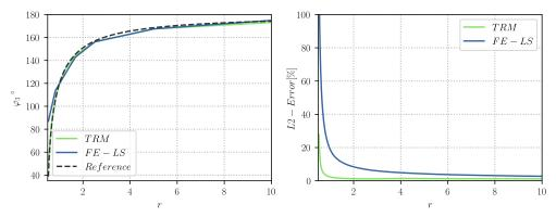
**Figure 5.** Triple junction test case: (**left**) Final value for the  $\varphi_3$  angle plotted against the grain boundary energy ratio r and compared to the analytical equilibrium value, and (**right**) L2-Error. The plotted data for the LS-FE model was taken from [8].
