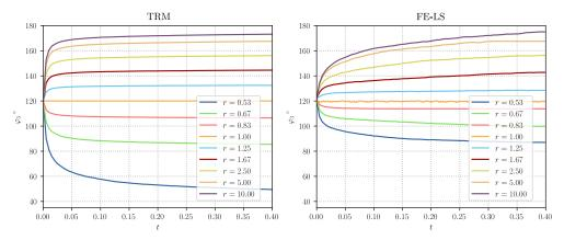
**Figure 4.** Triple junction test case: Evolution of the  $\varphi_3$  angle for different values of r, (**left**) TRM and (**right**) LS-FE models. The plotted data for the LS-FE model was taken from [8].
