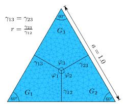
Figure 3. Initial state for the triple junction test: three grains are considered in an equilateral triangular domain. Dirichlet conditions  $\vec{v}_i = 0 \ \forall \ N_i \in \partial \Omega$  are considered in the domain border. The initial grain interfaces and the initial mesh are displayed.
