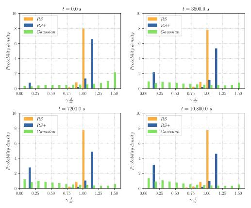
Figure 11. Normalised grain boundary energy distribution using various functions for the computation of the GB energy  $\gamma$ . The distributions are given for every hour of thermal treatment. Each class of data contains the results of four different initial states representative of the same initial grain size distribution.
